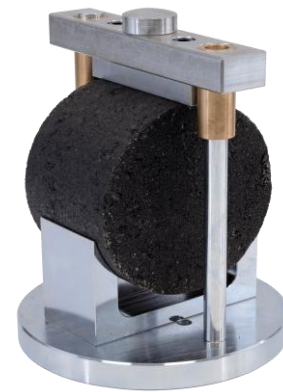
Figure 6. Typical IDEAL-RT Test Fixture [18]
