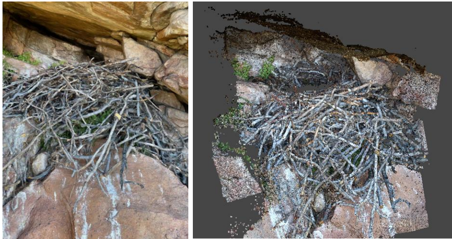
Figure 2. An example of imaging technology, differences in output, and imaging rates for a low-density fibrous composite (a raptor nest 200 feet off the ground). On the left is a still photo from a three-dimensional Lidar scan (which took under a minute to obtain) and the point cloud extension using SfM for the exact same nest but with 26 photos taken using a digital camera, which took about five times as long to obtain.
